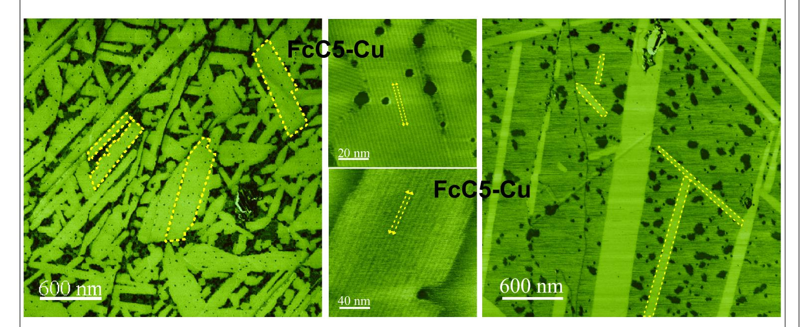
Facet angle ~ 85.5°; Spacing between link-like contrast ~ 6.8/ ~ 7.5 (FcC3/ 5-Cu) nm
