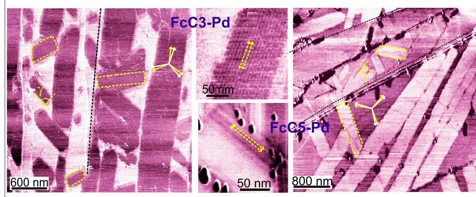
Facet angle ~ 84; Spacing between link-like contrast ~ 6.7/ ~ 7.5 (FcC3/ 5-Pd) nm
