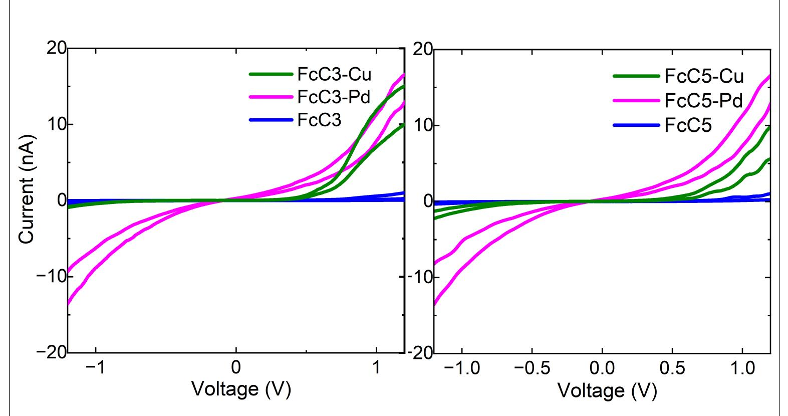
An enhancement in current of about 10 to 20 times upon doping; while Pd doping shows a symmetric I-V, Cu shows asymmetric I-V
