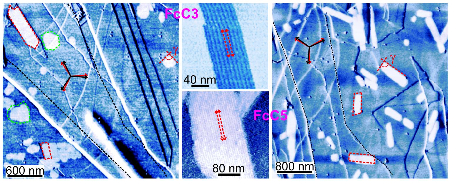
Facet angle ~ 83°; Spacing between link-like contrast ~ 6.7 (FcC3), ~ 7.4 (FcC5) nm
