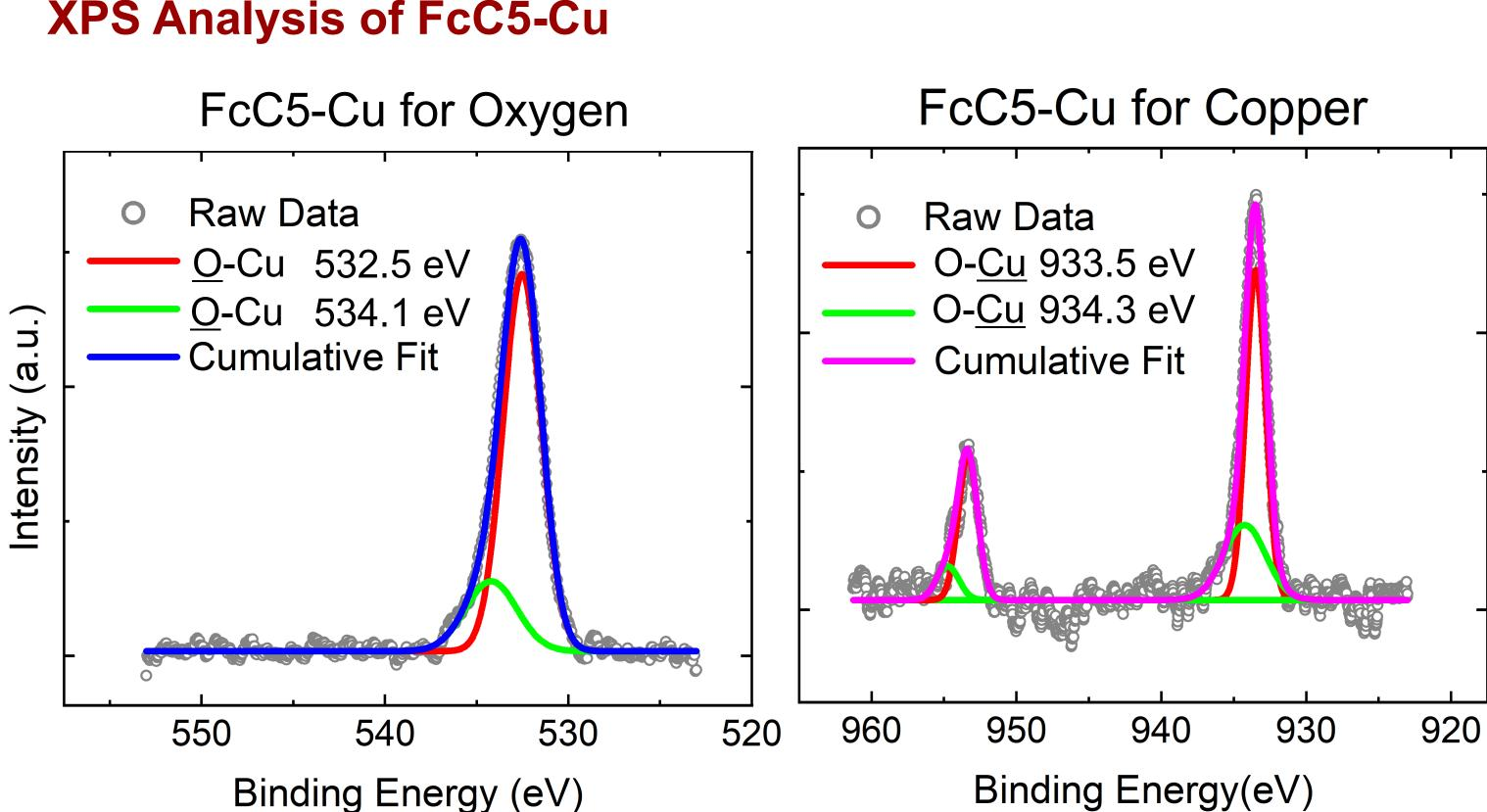
X-Ray Photoelectron Spectroscopy showing the binding with Oxygen and Copper
